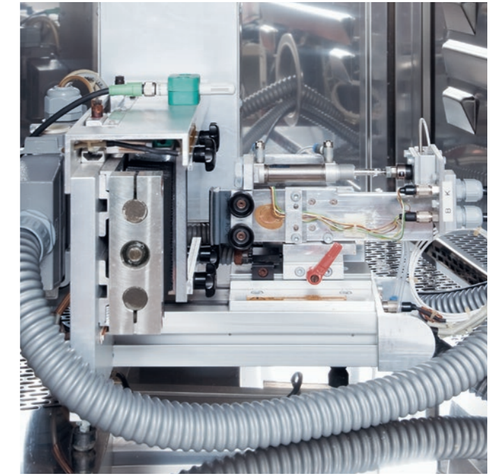
Stick-Slip test rig in climate chamber
