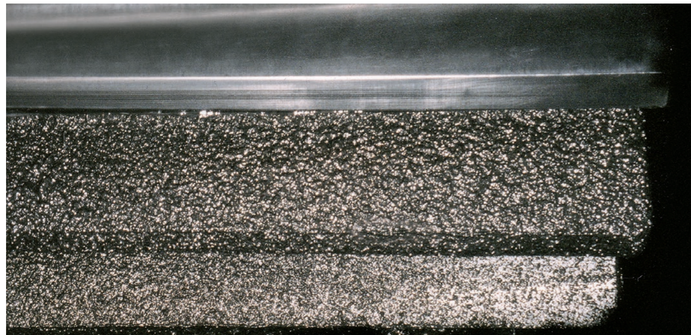
Berulit 443 in a sufficiently strong layer on the flanks
