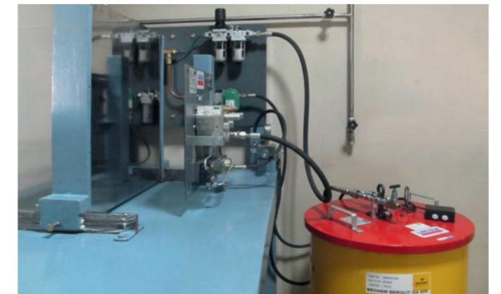
BECHEM has a spray testing system for adhesive lubricants to simulate customer-specific conditions
