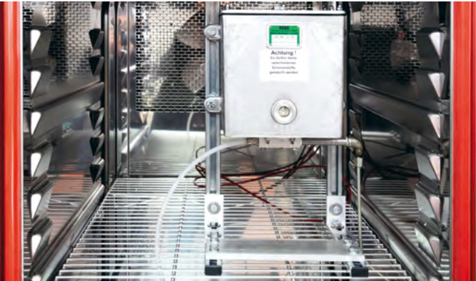
Test bench for wheel flange lubrication
