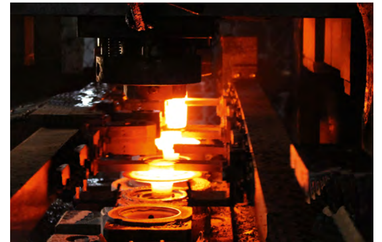
Berulit die spraying lubricants for optimised forging of automotive parts
