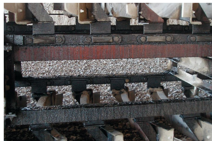
Sack palletizing: Use of Berulit IKP in chain lubrication
