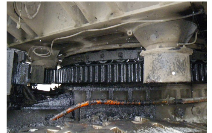
Slewing gear of a bucket wheel excavator lubricated with Berulit GA 2500
