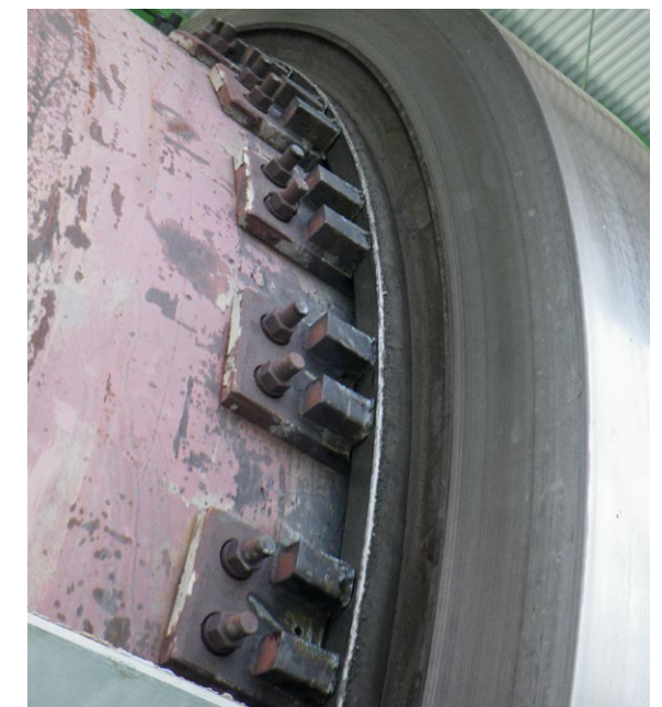
Well-lubricated tire at a rotary kiln
