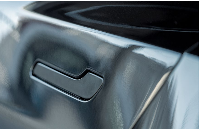
Door handles optimized for minimal wind resistance: Hydrophobic coatings can reduce the disruptive influence of water
